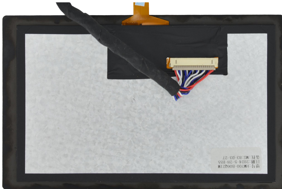
Figure 65 Connect LVDS screen cable to LVDS screen
